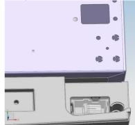
d. Screw off the 2 screws as shown below to remove the hole cover on the cabinet top, get the cabinet communication wire out of the hole; Pry up the small end cap cover on the door, and get out the door bush and door communication wire.
