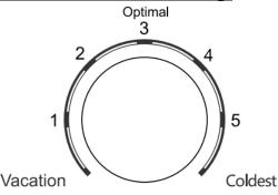
2. Adjust the refrigerator temperature setting will change freezer and refrigerator temperature together. For example, if adjust the setting from 2 to 4, both fridge and freezer compartments will get more colder.
