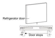
11. Install the refrigerator compartment door.
