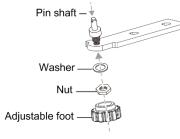
8. Install the lower hinge on the left side of the cabinet. Install the adjustable foot at the right.
