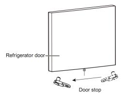
Install the refrigerator compartment door.
